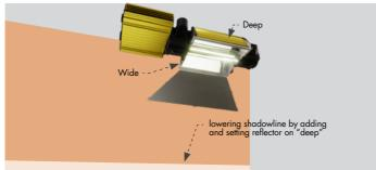
When the side-reflector is moved to the outer position, the reflector is in "deep" position, when moving the side-reflector towards the lamp, the reflector is in "wide" position.
